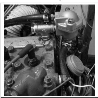
The traditional sensor opening in the head is now an excellent place to install a high temperature alarm such as the Cole Hersee Model COL-M40177BP.
